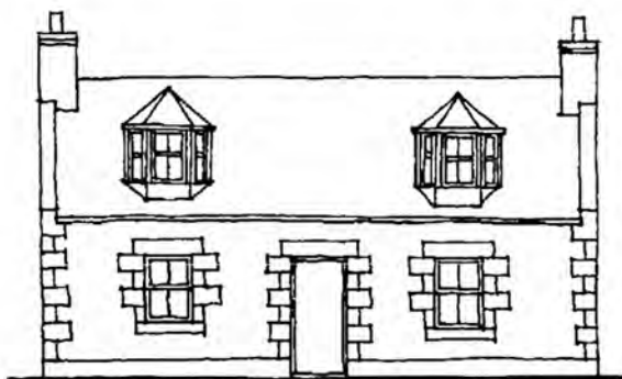
An example of how roof dormers should be positioned to be respectful of a building
