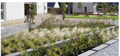
More structured and formal 'rain gardens' which gather and hold storm water during events and slowly release water back into the environment in a controlled rate.
