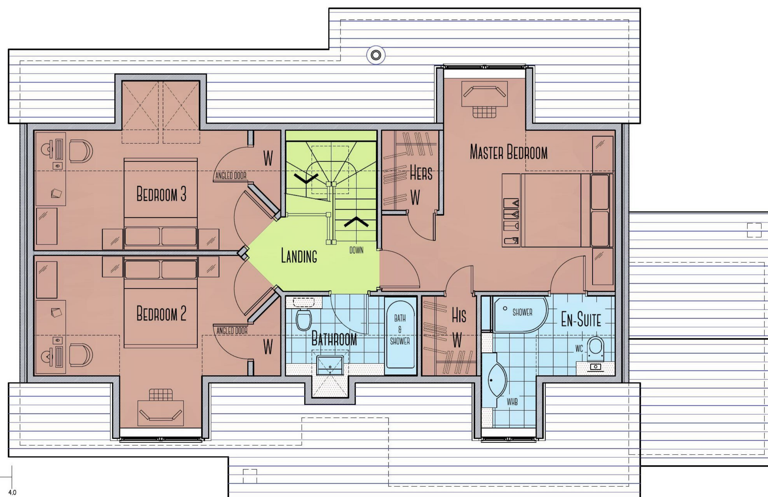
PROPOSED FIRST FLOOR LAYOUT PLAN SCALE 1:50 @ A1 FIRST FLOOR G.I.A = 72M/SQ OR THEREBY
