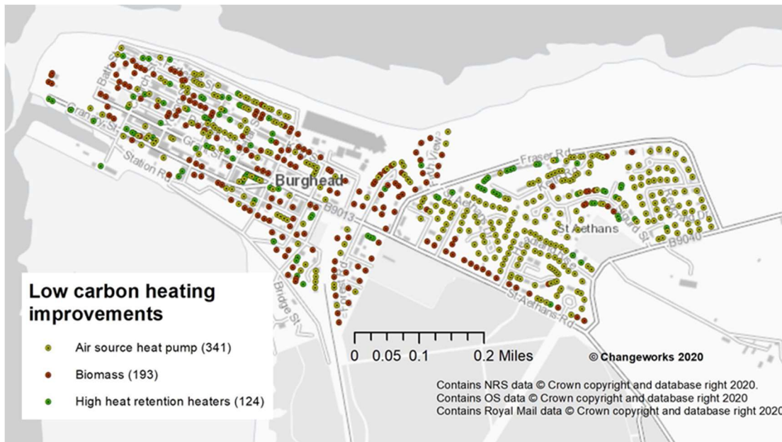
Figure 6: Low carbon space heating upgrades (Burghead)
