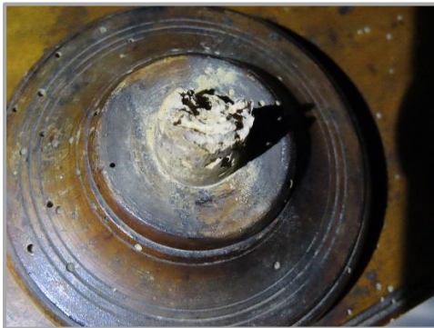
Dust around damaged spindle
