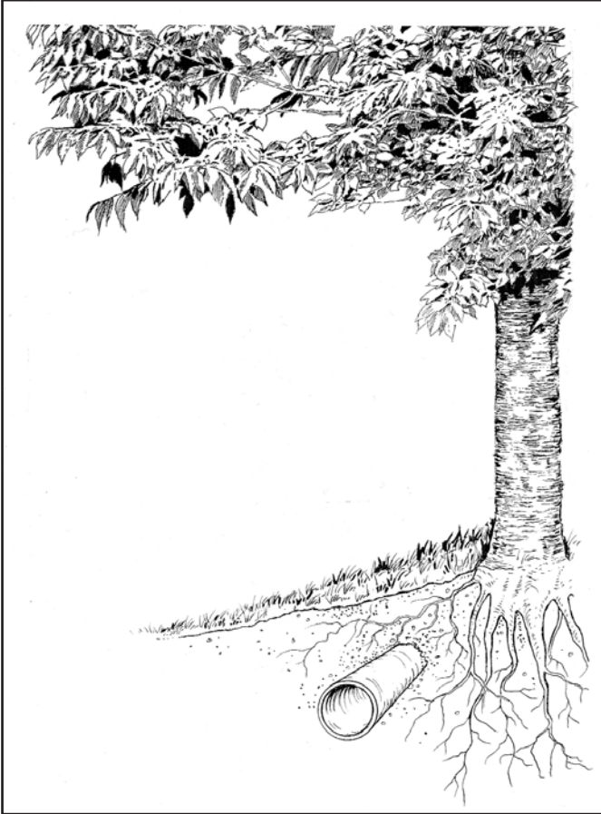
Fig 2: Invasive root systems minimised by tunnelling utilities under the tree.
