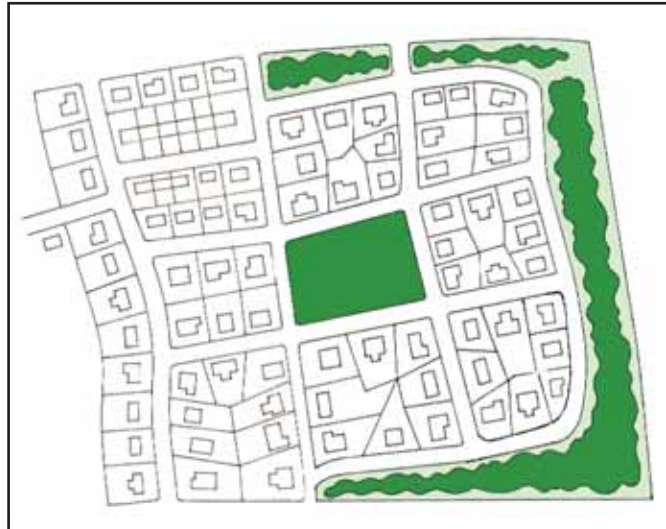
Perimeter block layout with central open space
