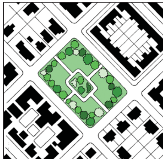
Perimeter block layout with central open space
