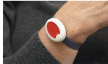
The personal trigger will raise the alarm if pressed anywhere in the house. It is completely waterproof, so it can be worn in the bath or shower.
