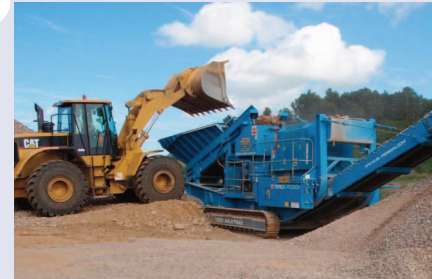
On-site crushing operation to re-use waste material
