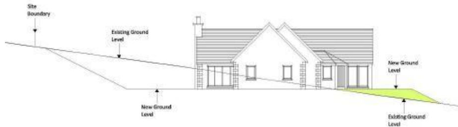
site section – shows proposed house cut into slope of site to east
