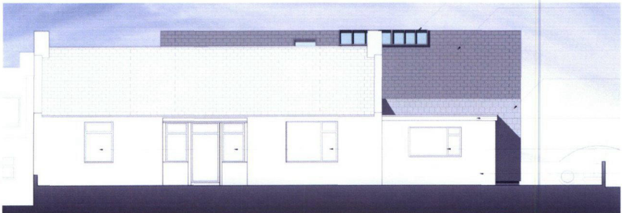
Image 26. West Elevation of existing fisherman's cottage in foreground, & the proposed homogenous slate roof & wall to the rear
