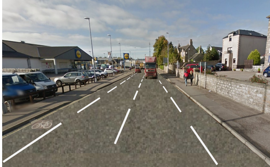
Station Road, centre turning lane removed and cycle lanes added.
