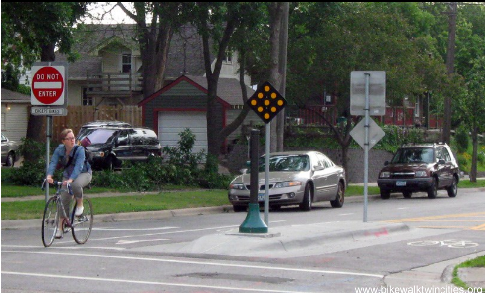
RiverLake Greenway (40th Street), Minneapolis, Minnesota. Drivers approaching this junction from both directions are forced to turn, but bicycles may continue straight.
